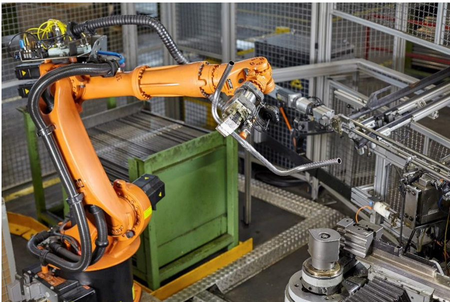
picture: Handlebar bending with the Kuka robot
